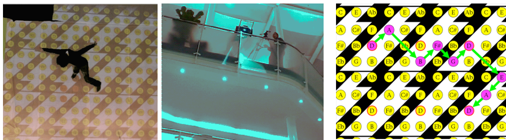
Figure 1: left – a player throwing shapes in the Harmony Space representation projected onto the floor; middle – a projector on the top floor of the atrium, with two metal arms holding a mirror for downward projection; right – the path of the chord roots of Pachelbel's Canon in Harmony Space.
